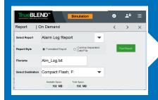
Built-in reporting Every SB-5 blender control is equipped with the capability to help users track their settings, alarms, material consumption, shift and inventory needs.
