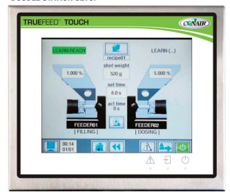
The new TrueFeed Touch allows you to view and control both feeders on the same screen, simplifying work with multiple feeders.
