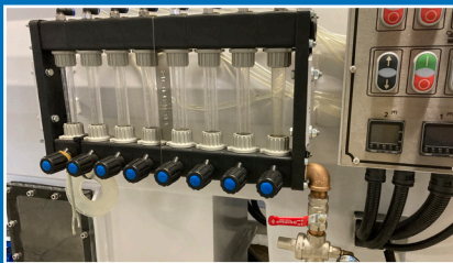
Water flow meters
